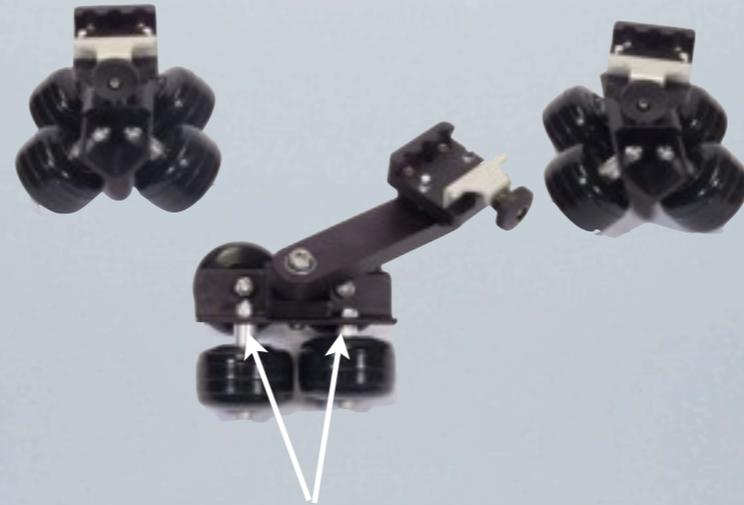
Note that 2 of the 4 wheels per cluster are spaced out differently. These wheels are primarily intended to be used on track. However, because they are spaced out like this, when they are placed directly on the floor, only 2 of the 4 wheels touch the floor. This allows the dolly to roll on the floor which it could not do if all 4 wheels were touching. This feature is usually used simply to reposition the jib. To actually do an in-camera move you would need to be on a very smooth floor.
