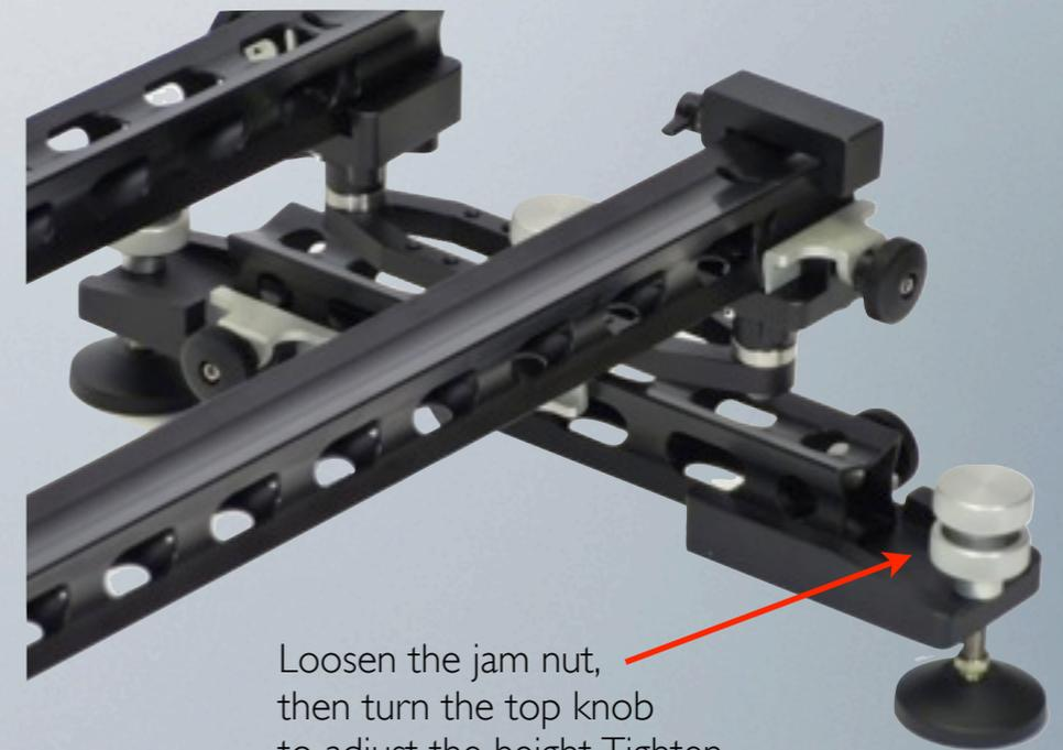
Loosen the jam nut, then turn the top knob to adjust the height. Tighten the jam nut when finished.
