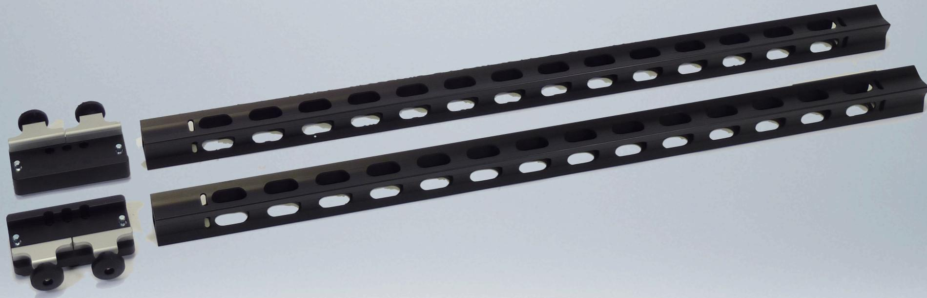
We recommend not exceeding 6 feet between support points, however for this 9 foot assembly you actually do not need any more supports. You simply move the tripod support in approximately 18 inches from one end, and the monopods in 18 inches from the other end. Now you have a 9 foot run, but still only a 6 foot span between the supports. The short 18 inch overhang on each end does not need any additional support. Of course, to go to 12 or 15 feet , or more, you will need more supports.
