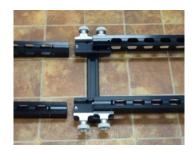
1) Place cross braces and rails on floor and clamp together. Make sure the spring-loaded locating pins engage into the slots on the rails. Tighten the knobs securely to make sure the rails align.
