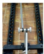
4) Add the long turn-buckles to the under-carriage supports. The two end section rods are slightly longer than the center section rods. You may need to fine tune these once the system is upright. If the turnbuckles have been over-tightened, the trolley may run rough.
