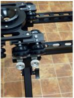
7) Temporarily remove endstop, and slide trolley onto the rails.
