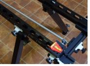
6). Use end-stop clamps with bubble levels to set level. although a carpenter's level is better for checking if there is any sagging in the middle. Height can be set by telescoping the legs, or by changing the angle of the legs. Once the legs are set, make sure upper and lower leg locks are tight.
