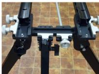
9) For additional lateral support, move undercarriage clamp over and add a third monopod to each end.
