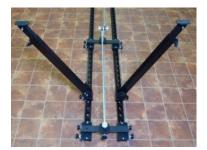
5) Add a set of 2 monopods near the end of each rail (in approximately 12" (30cm.) from the end. Then turn the assembly right side up. If working alone, lift from the center point of the assembly.
