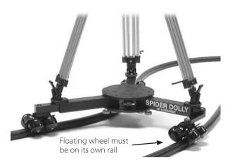
Slowly roll the dolly over the track while watching the floating wheel and adjust either rail in or out as necessary (nudging with the foot) so that the arm tracks directly over the rail. Watch that the articulating arm does not move all the way in to hit the mount, or all the way out to be perpendicular to the rail. Either situation will result in a mis-track and prevent smooth movement.
