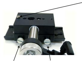
This small screw can act as a locating pin for certain quick release plates that have only one tie-down screw, (smaller Cartoni heads, for example). However, some plates have a slot too narrow for this provided locating pin, (Manfrotto for example), so you will need to remove the small screw pictured here, and use the two-screw method.
