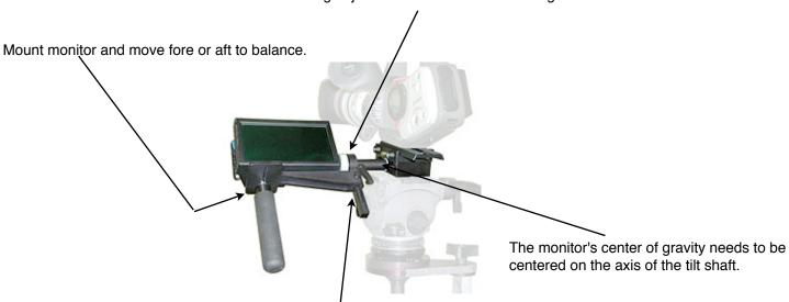
Loosen Kipp lever, and raise or lower monitor to balance. Turn monitor 90 degrees so that it is parallel to the ground to more easily determine the balance point.
