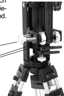
5) Loosen the lever that clamps the 3" main tube (at the upper end of the assembly).
