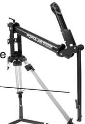
8) Slide the T-shaped end of the Secondary Arm into the guides located on the inner sides of the main upright supports. Secure by inserting the through-shaft and knob you removed in step 4. Lock the lever that clamps the 3" diameter main tube (the clamp loosened in step 5).
