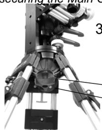
3) Position the Traveller onto the 100mm bowl of your tripod or dolly. From below the 100mm bowl, connect the Traveller to the tripod with the tie down knob and 2" washer.
