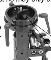
Thread the 3/8-16 rod into the base of the Traveller.
